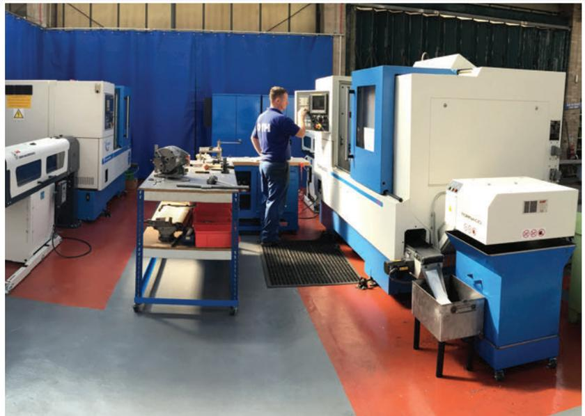
Ever seeking new technology, DTH has further invested in two Tornado 3 Axis CNC Barfeed Turning Centres with the intention of supplying new and existing customers with multiple quantities of products in various materials up to 80mm diameter.
